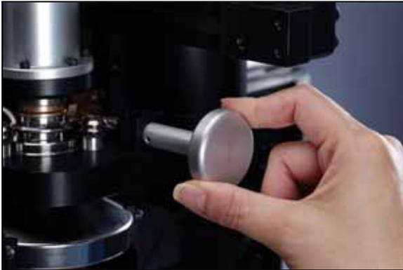
The lower heater head can be rotated by turning the Theta Adjust knob. This rotates the nozzle and the vacuum pick-up, so the component and/or nozzle can be aligned to the PCB in the Theta, or rotational, direction. The Theta adjust is a precision assembly with limited travel in either direction. Take care not to continue to turn the knob once the Theta has been adjusted to the end of travel to avoid damaging the assembly. (Also see: Nozzle Installation)
