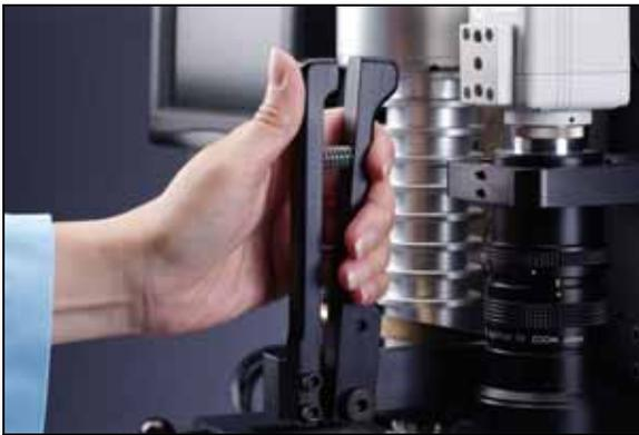
Figure 13: Z-Axis Adjust Handle
