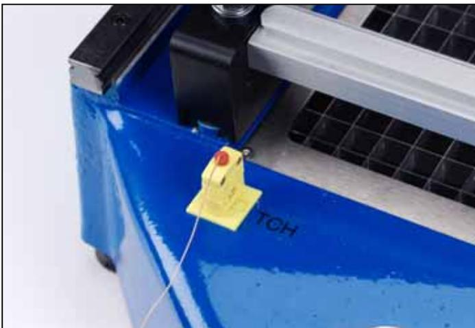
Figure 6: Thermocouple Inputs (TCH Shown)
