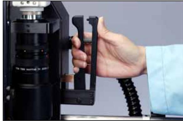
Figure 9: X-Axis Adjust Handle
