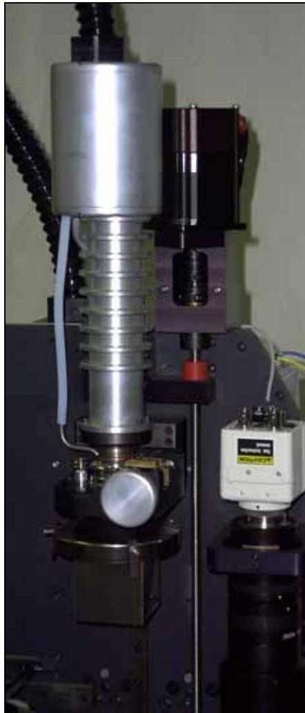
Figure 29: Automatic Motorized Z-Axis Option
