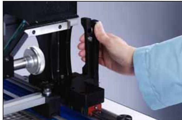
Figure 11: Y-Axis Adjust Handle
