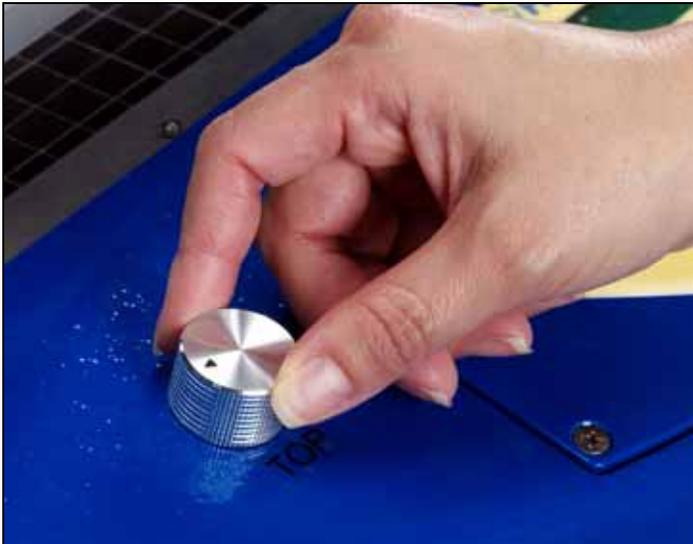
Figure 4: Lighting Intensity Control
