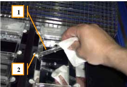
Figure 33: Replacing the bottom heater quartz lamps
