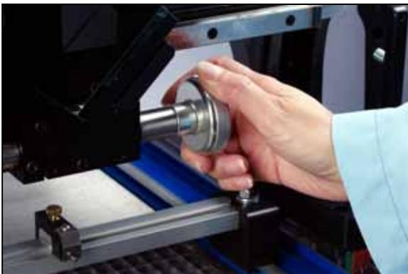
Figure 14: Z-Axis Fine Adjust Knob
