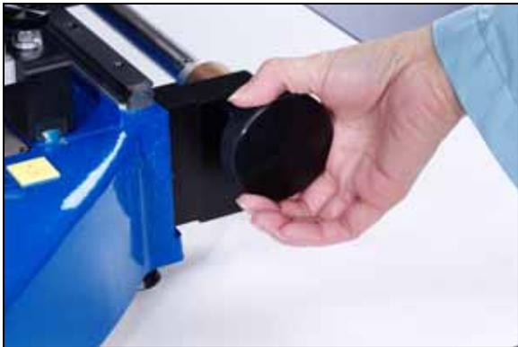
Figure 10: Y-Axis Fine Adjust Knob
